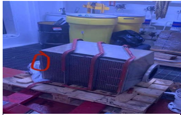
EGR cooler with location of weld failure indicated
